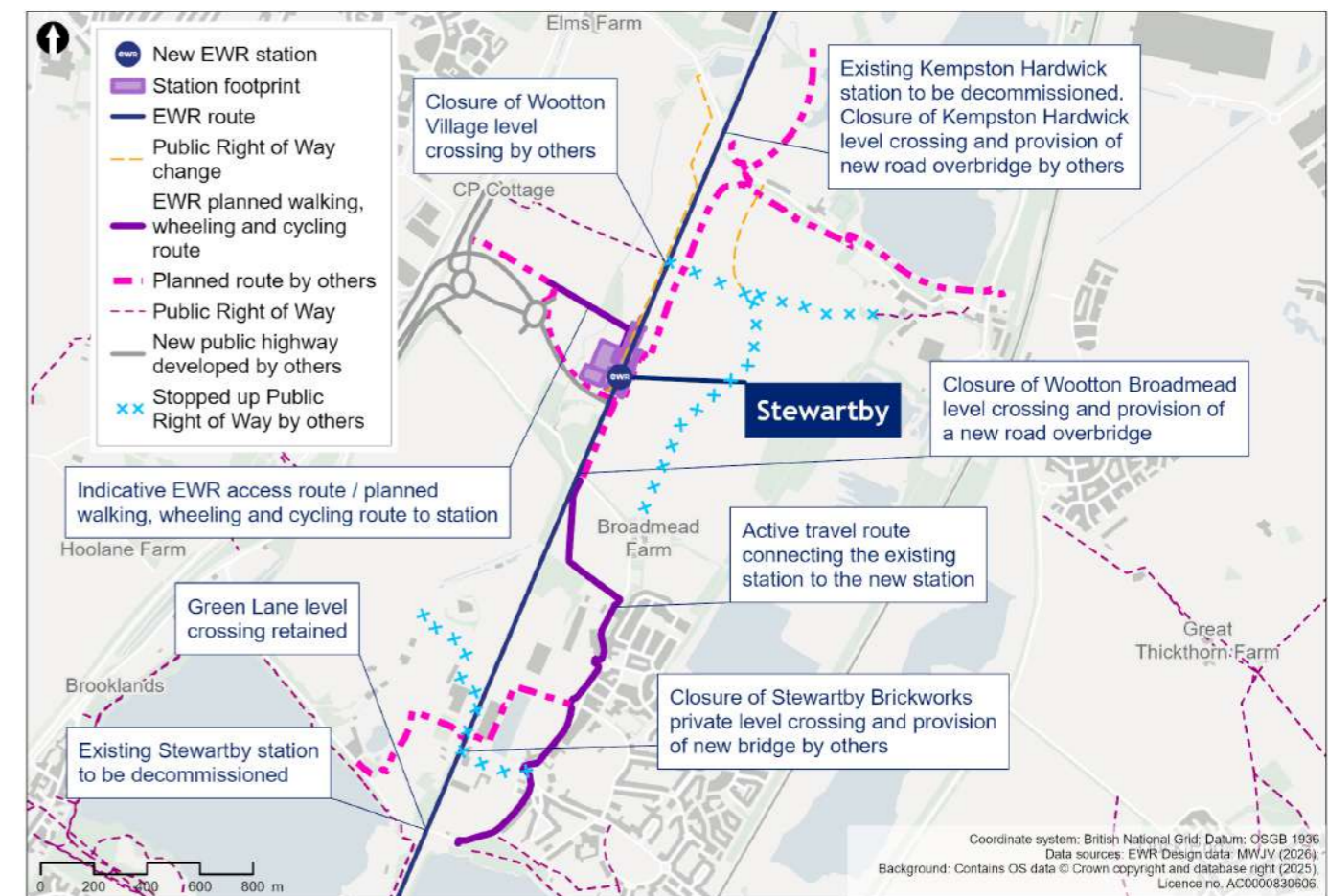
Figure 47: Map showing our proposals for level crossings around the new Stewartby station
