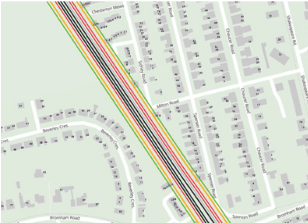
Figure 8.20: Six Track Western Variation A indicative track positions in reasonable worst-case railway corridor width
