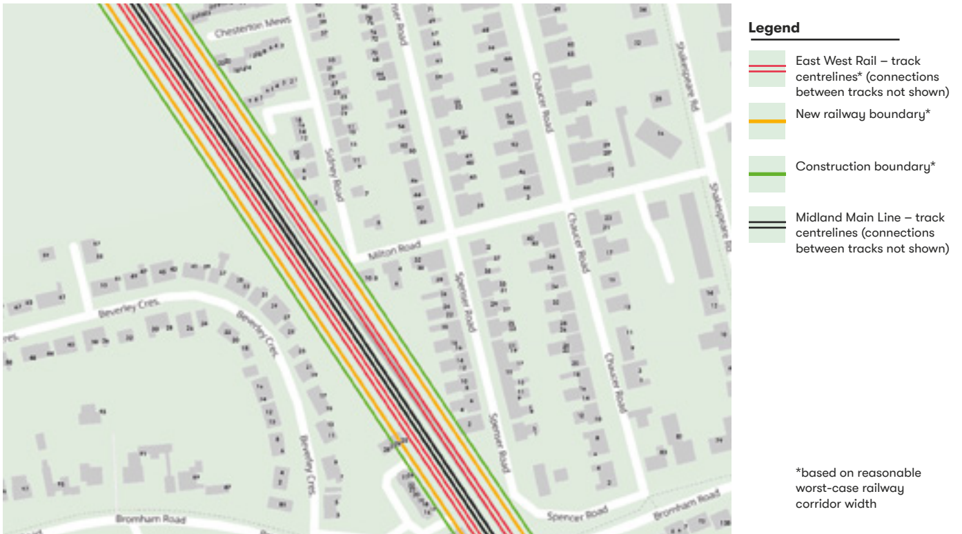
Figure 8.19: Six Track Western indicative track positions in reasonable worst-case railway corridor width
